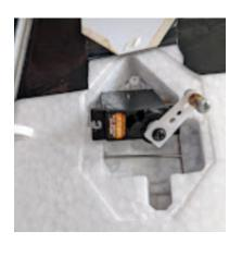
From the "cover" image - had a substantial crash? While you're making more obvious repairs, remember to also check for more hidden damage, including the condition of servos, motors, and other electronics. While gluing up wing and body damage on an Eflite Timber, yours truly found a stripped flap servo on the broken side of the wing.
