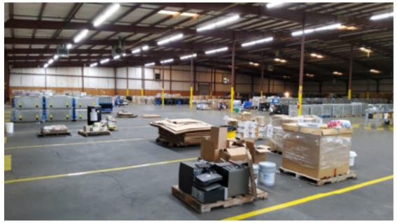
This facility is an EPA Responsible Recycling (R2) approved vendor called Battery Recycling Made Easy, in Norcross, Georgia. There, BRMS shreds and hammermills the batteries resulting in what they call "metal concentrates" that are then used for alloy production. Circuit boards, if present, are forwarded to ITAD Technologies, an electronics recycler.
