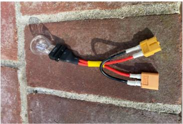
This smoke-stopper can also function as a load to slowly discharge a battery. All that is required is to plug one connector in to the battery, and then to complete the circuit through the other connector. For this, I built a simple loop connector that just shorts the positive and negative poles of the connector.
