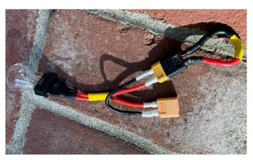
This one is suitable for discharging up to a 3S LiPo (it's a 12V bulb). The battery needing disposal was a 4S, so I connected two such smoke-stoppers in series.
