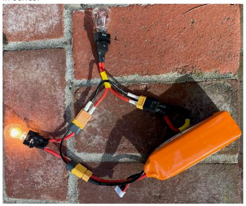
Once I'd let that sit for several hours, and the voltage was reading near zero (about 0.1V-0.2V), I just plugged my short-circuit connector directly in to
