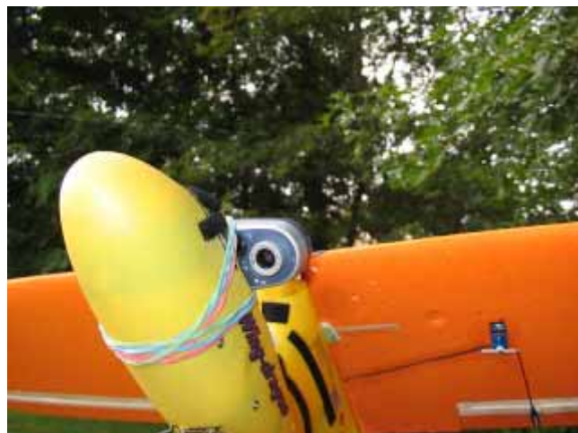
Aiptek 1.3 mounted on brushless WingDragon.
