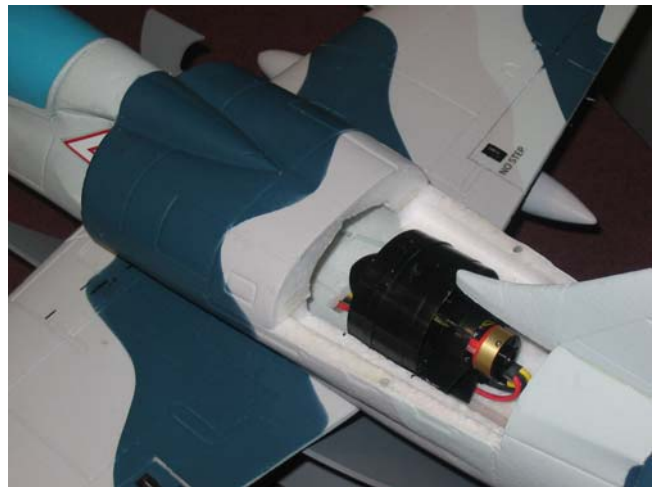
Hyperflow Fan with Ammo 4850 brushless in-runner
