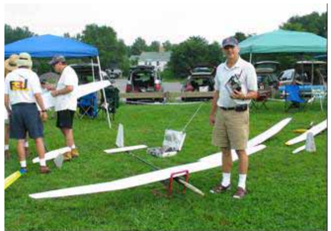
Anker Bergson stands by his Supra sporting his own wing and tail groups. Anker is producing Supra wings and has just installed a CNC foam core cutter. This is the first production wing. Each run looks better and better.
