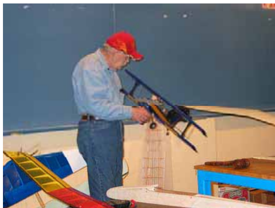
Bill Johnson displayed his Ultimate Biplane, an Ace kit. Bill has installed a 480 brushless outrunner, coupled with a 10-5 prop. The plane has both wheels and floats, and weighs just under two pounds.
