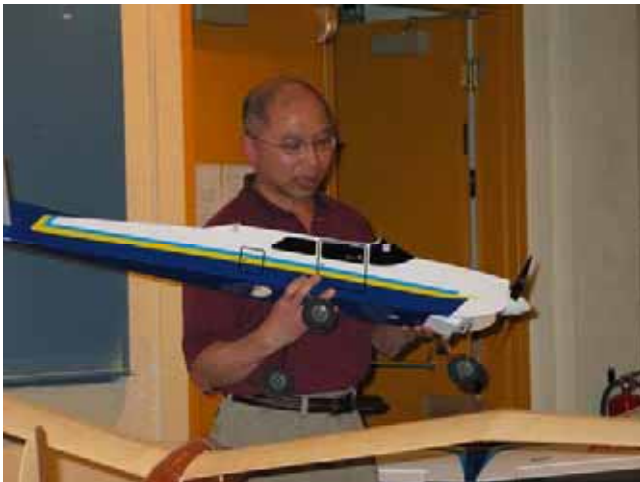
Stephen Young's German Alula EPP HLG came with a twist in the wing. Stephen used his wife's hair dryer to successfully remove the twist, but worries that the wing will return to its former shape in heat of the summer. The Alula has a 34-inch wing span and weighs 120 grams.
