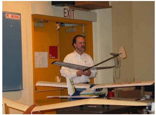
Dick Williamson completely rebuilt his Bird Of Time after folding the wing last summer. Dick is the third owner of this classic sailplane, and estimates the plane to be 30 years old. The wing collapse resulted from a failure in the brass tube wing joiner. Dick added carbon fiber to the top and bottom of the wing spars, beefed up the wing rod, wrapped the spars in Kevlar, and added spoilers. A new covering finished the job and it looks just like new. Dick reports that his BOT flew straight and true during a recent visit to Davis Field.
