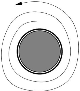
Spiral wrap with 1" wide 1 mil polyethylene strip
